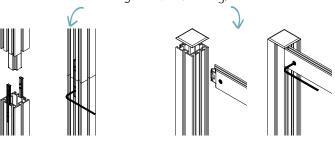
Linear profiles can be connected using a connector system already integrated into the profile.
