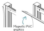
Rigid panel graphics (5mm) allow the panel to fit directly into the channel of the post. If you wish to cover the entire structure, male and female hook and loop fasteners are used on the back and on the structure.
