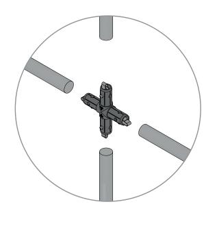
1 Assemble the corners using the mounting brackets and assembly markings.
